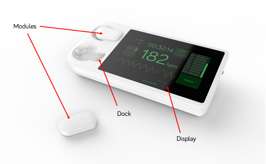
Figure 1-2 Display with Modules. There are two Docks for charging and storing the Modules.
