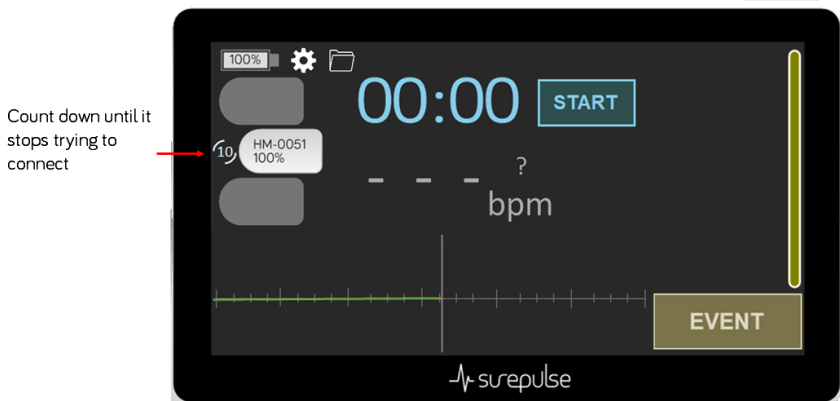
Figure 3-16 The Active Module is trying to connect. There is a count-down timer for the connection attempt. If the connection attempt fails, replace the Module in the Display and try another Module.
